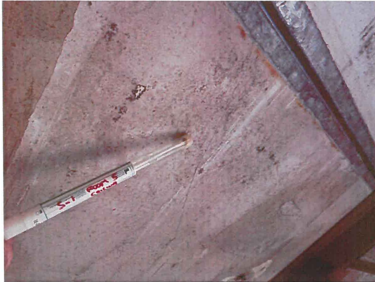
Mold Surface Sample S-1 – Classroom #5 Ceiling
